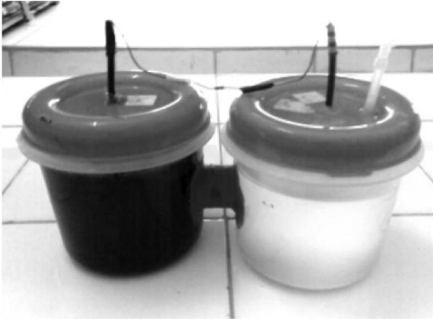
Arboleda constructed several of these makeshift MFCs using simple materials to test the power generation potential of several substrates
