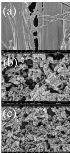
The electrographs from the scanning electron microscope show regular filter paper (top) and filter paper with copper particles (middle and bottom).
